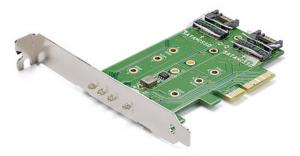
This 3-port M.2 SSD adapter card is one of the only cards that supports both PCIe and SATA-based M.2 SSDs (solid-state drives). It's a versatile way to expand the overall storage capacity of your desktop PC or server. Plus, because it supports a high-speed PCIe M.2 drive, you can increase the speed and performance of your computer.
